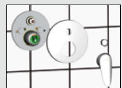
Slide the plate support over the cartridge and the diverter and screw into the right position. Then mount the visible design parts.
